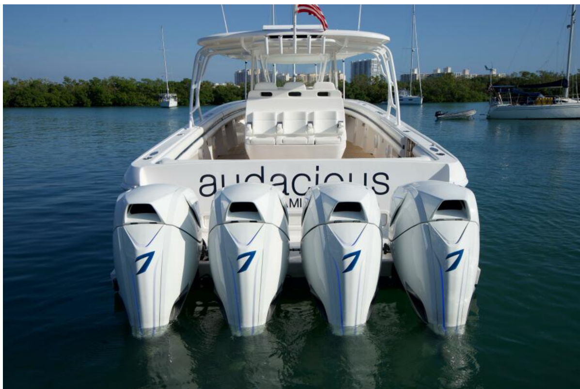
ENGINES 47' (14.33m) Intrepid, 475 Panacea, 2016 - (4) Seven Marine 627 SV Dual Prop (627 HP)
