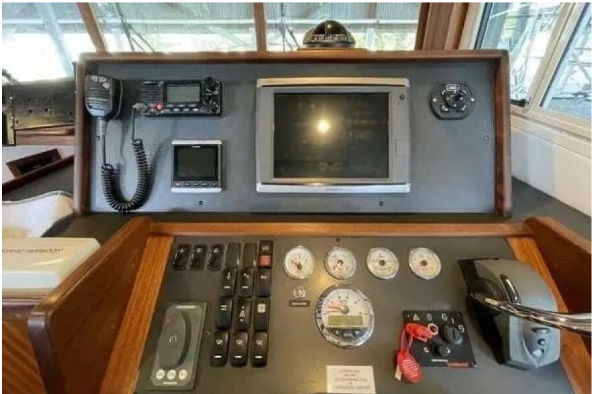
Helm/electronics Garmin 7212 Multifunction display Garmin GMR 18 HD Radar Garmin GSD 22 depth sounder Garmin GHP 10 Autopilot Garmin GHC Autopilot control Garmin AIS P79 in hull transducer Jabsco remote spotlight Horizon VHF Fusion marine stereo Shakespeare VHF Antenna
