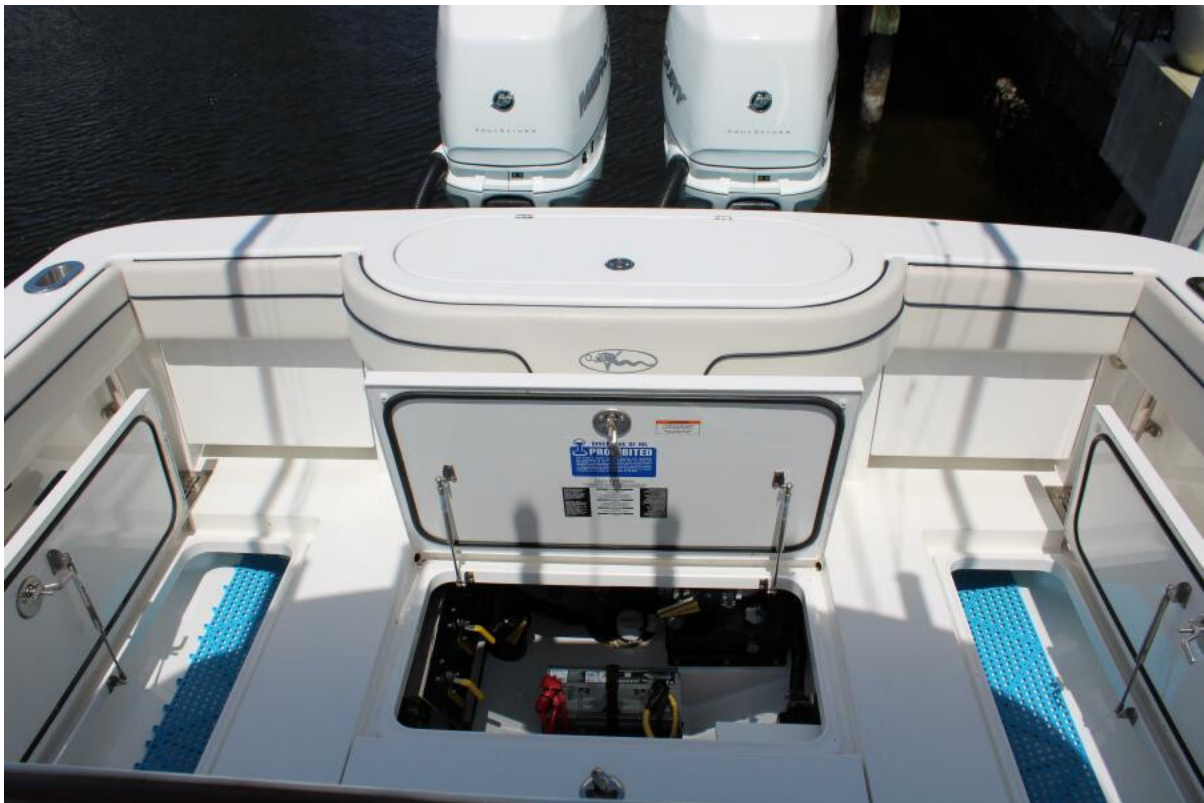
Deck Access to Batteries, Port and Starboard In Deck Storage
