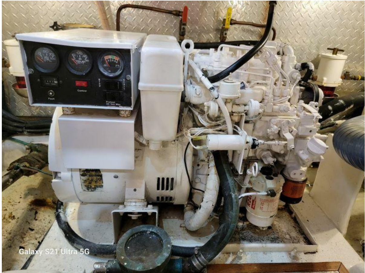
40' Marine Trader Onan 8kw Generator
