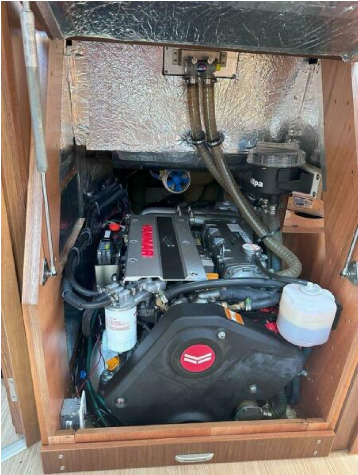
Engine, 80 HP Yanmar
