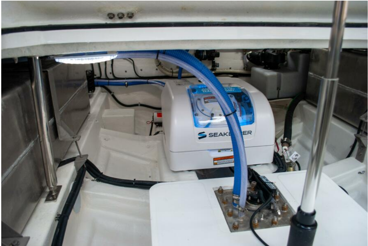
Seakeeper 1 gyro stabilizer removes 93% of boat roll
