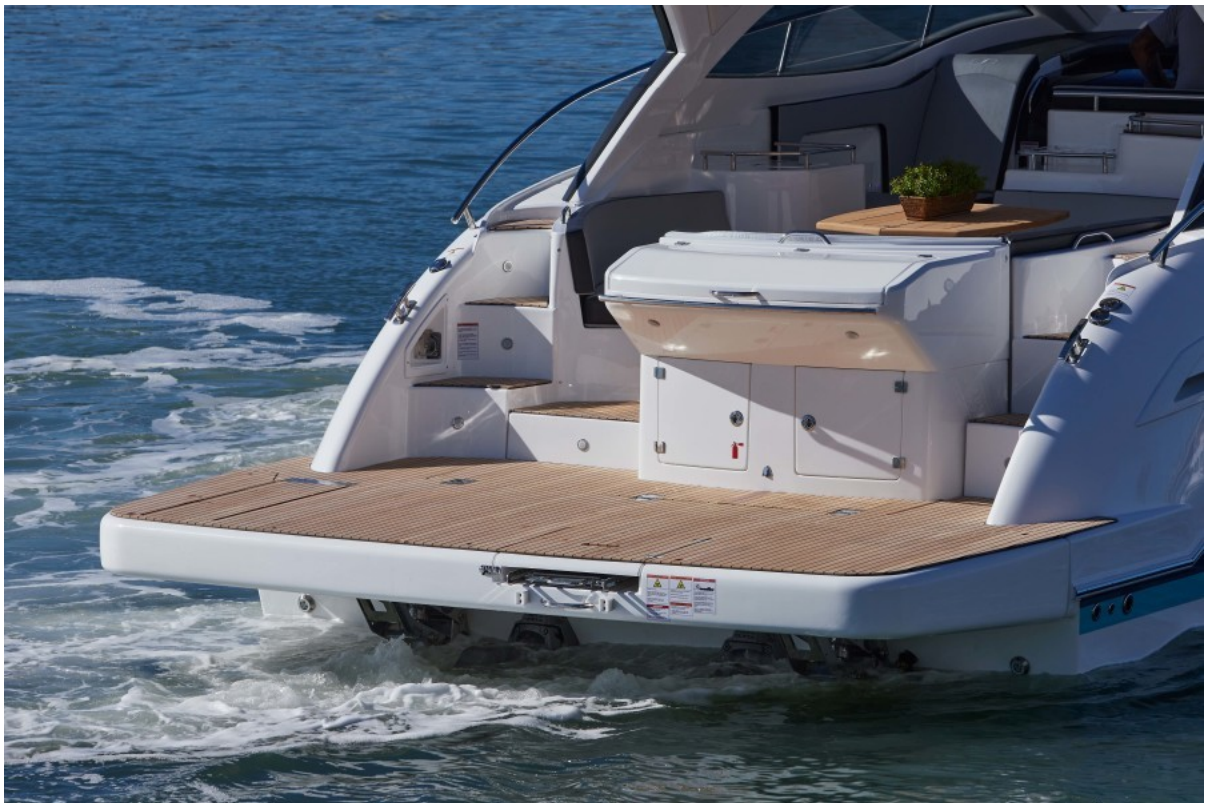
Swim Platform Large hydraulic swim platform is available with disappearing steps
