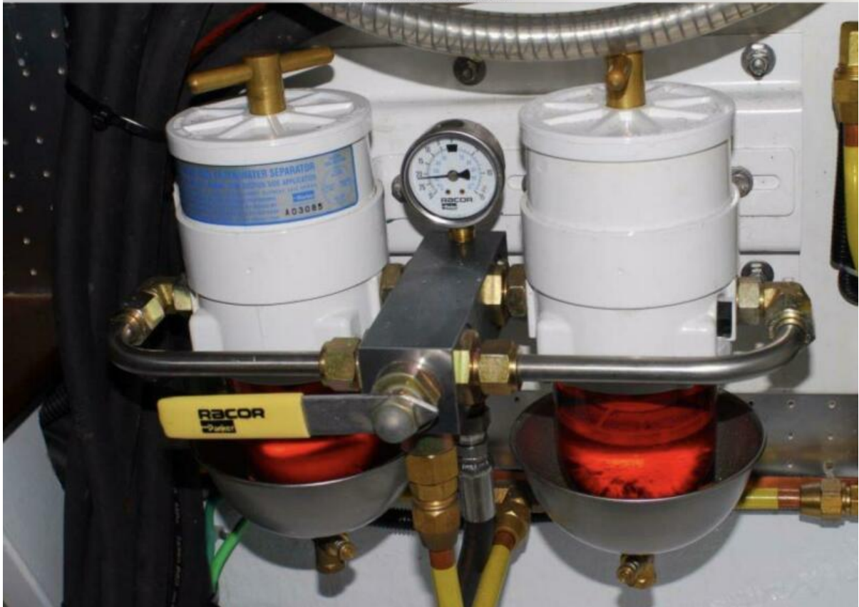
Dual Racor Fuel Filters
