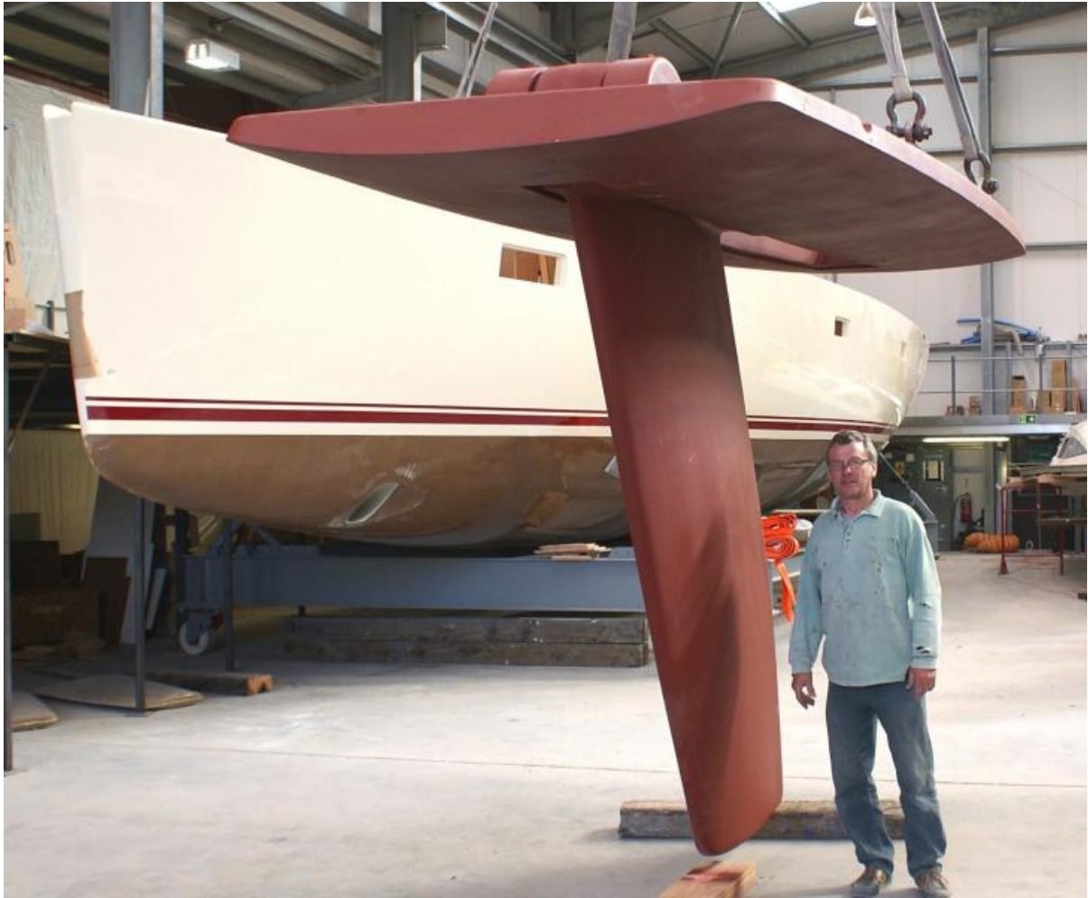
Southerly Swing Keel Grounding Plate: 11,749 lbs Swing Keel: 7,385 lbs
