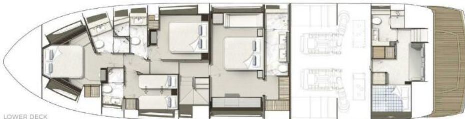
LOWER DECK Shown with optional sliding inboard berth in port guest cabin. Optional engine room access door and optional Pullman bunk in aft cabin
