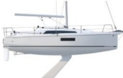
Profile - Lifting keel version
