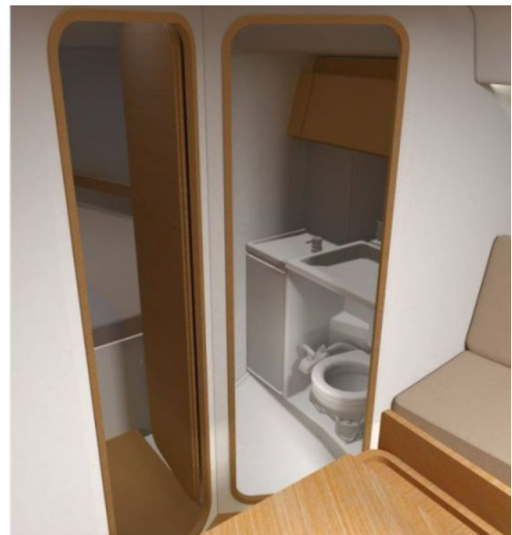
• Big pivoting sink to free up space • Mock-up tested layout for optimal size • Integrated Shower Water tank Free rotation of shower head allows wide flex Storage cabinet with mirror head (space for feet) Plumbing kit Shower head Modular storage unit Toilet seat made from recycled GPP for efficient water Toilet seat (recycled GPP) Shower cabinet (space for feet) GPP part 85 cm 45 cm 50 cm
