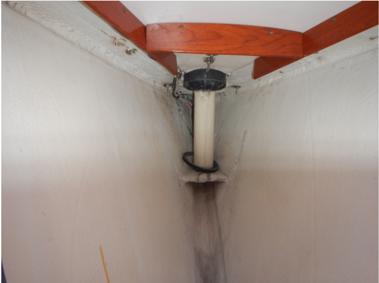
Dislocated Hoyt Boom Interior Bushing
