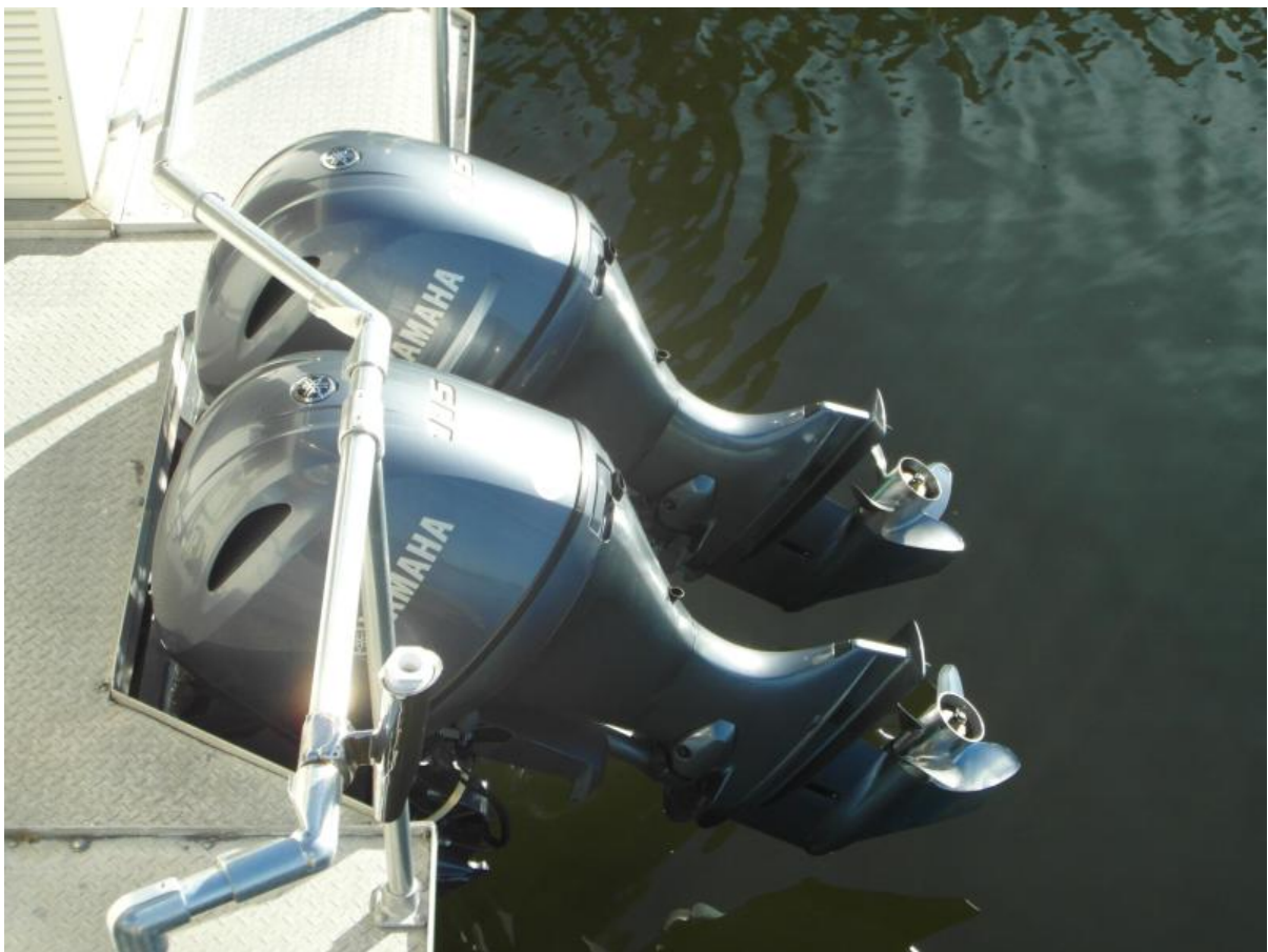
2006 Trident 44 Passenger Tour Boat Hydraulic Rotating Jack to Raise and Lower Engines
