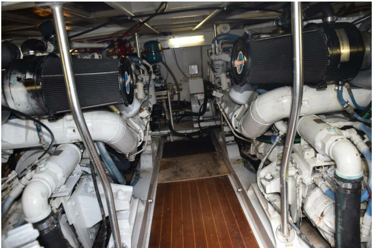
Engine Room, Detroit Diesel 8v92s
