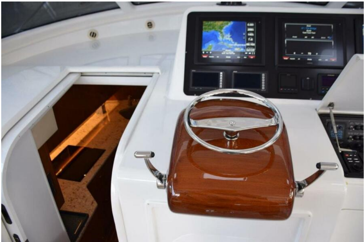
Teak Helm Pod with Thruster Buttons on Levers
