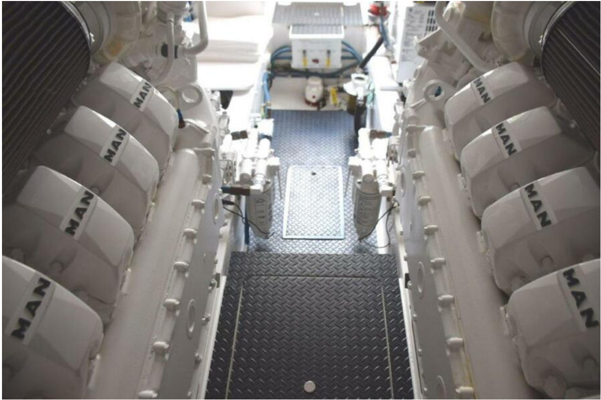
12-Cylinder Common Rail MAN 1400HP
