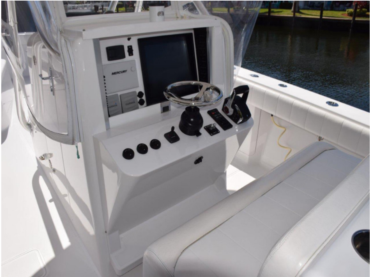
Panel cover slides down to disappear when open
