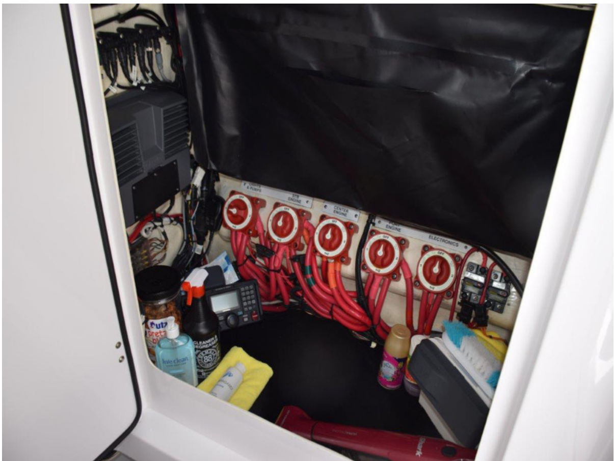
Battery switches and access to console equipment
