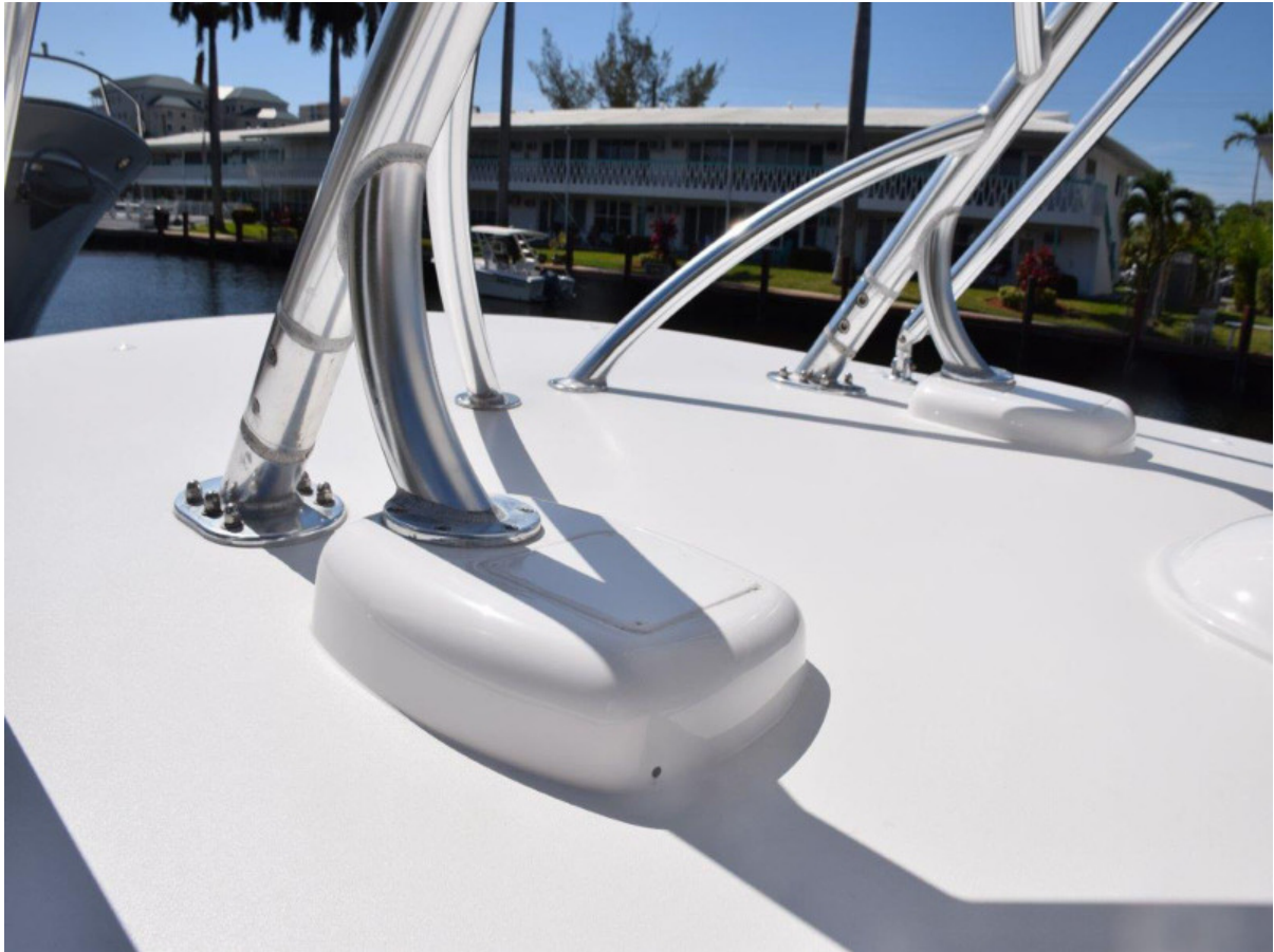
Tower can be removed with quick connects
