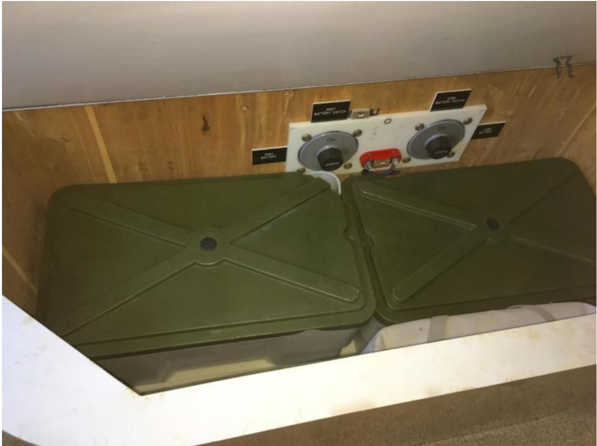
Batteries under aft bed and port engine access
