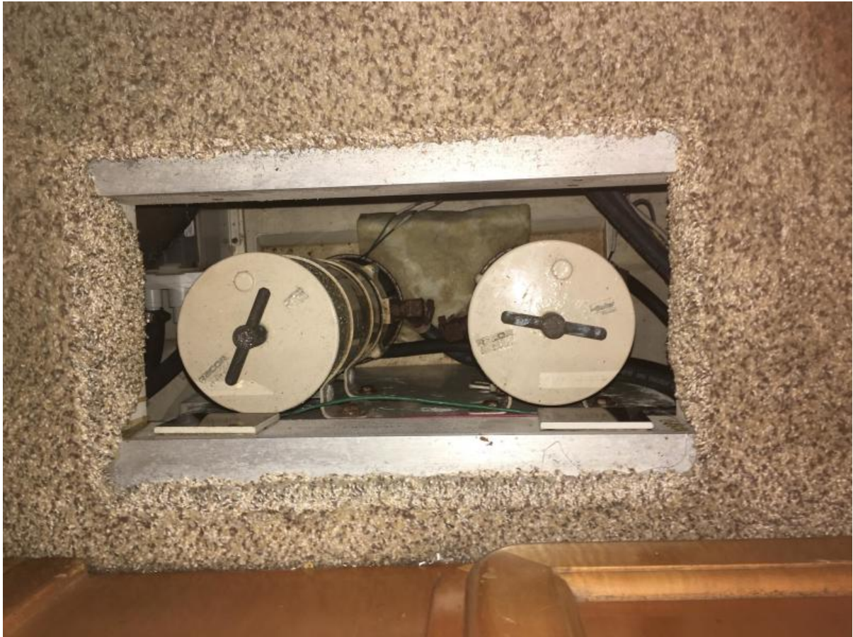
Racor dual filter in floor locker
