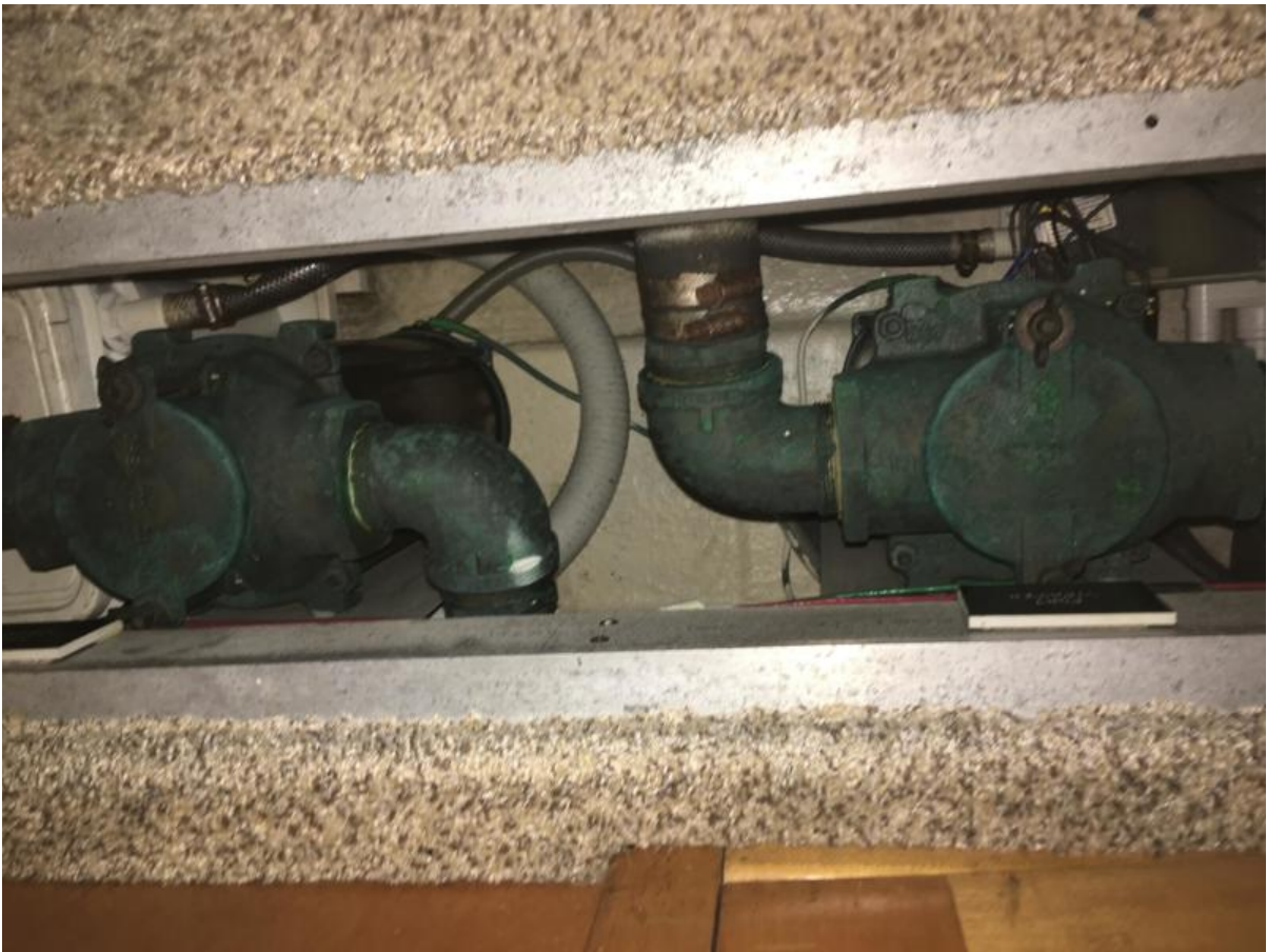
Raw water filters in floor locker
